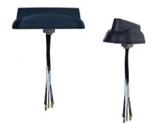
The Gar VFP69383B22JN multiport/multiband antenna provides an excellent solution for Public Safety, Transportation and Aftermarket Fleet applications. Configured for 2-port MIMO operation over the 3G/4G/5G/ISM/CBRS bands and 2-port MIMO operation over the low//high frequency Wi-Fi bands. An additional 5<sup>th</sup> port provides an active antenna for enabling GNSS global navigation services.
