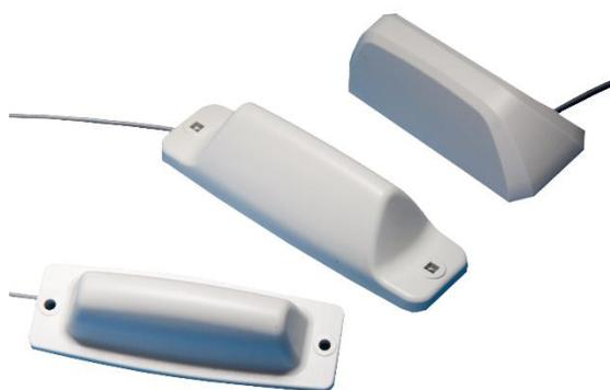
LP80x series antennas offer ground-plane independent Omni-directional performance with discreet and durable design. The low profile housing gives a high degree of vandal resistance making it perfect for smart meters, tracking devices, vending machines and other M2M applications, where it requires reliable communications.
